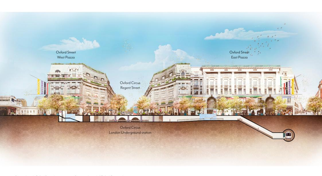
Section through Oxford Street showing two new Piazzas either end of Oxford Circus with improved access and new entrances from the piazzas directly into the underground station.
